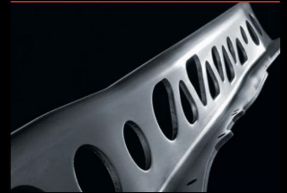
Drivetrain twist wastes power and produces acceleration lag. To help eliminate that, Mazda engineers gave the MX-5 a solid structural “backbone”—an ingenious aluminum Power Plant Frame that unites engine, transmission and differential into a single rigid unit.
