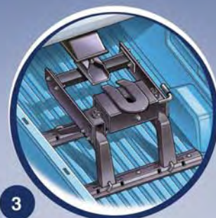
2 Fifth wheel kingpin fails to seat properly and slips off the hitch.
