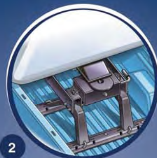
1 Fifth wheel hitch with BedSaver™ in place.
