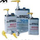
resin and hardener containers and eliminate the mess involved with measuring by weight or volume. 300 Mini Pumps are calibrated to deliver the proper working ratio with one full pump stroke of resin for each one full pump stroke of hardener. Set contains one resin pump and two hardener pumps.
