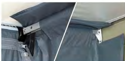
The ends of the Buena Vista lock up tight against the vehicle and the roller without drilling or permanent mounts.
