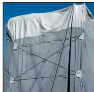
Attached Nylon Straps & Plastic Buckles Hold Cover in Place
