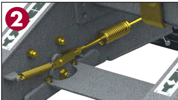
Truck moves forward, compression cylinder relaxes to allow flipper to work
