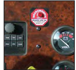
BrakeMaster LED An LED in the motorhome provides a visual reference of braking activity.
