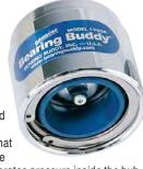
grease which generates pressure inside the hub to keep water out. If the lubricant is low, the blue Auto Check ring will recede until it is flush with the steel-retaining ring. Add a small amount of grease to move the blue ring outward about 1/8". It's that simple! Fits outer bearing cone numbers: L44643, L44649, and L44640.
