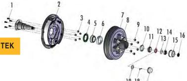
AXLE TEK, DEXTER 12" x 2" HUBS-DRUMS AND IDLER HUBS, 6 ON 5.50 BC 5200# & 6000#
