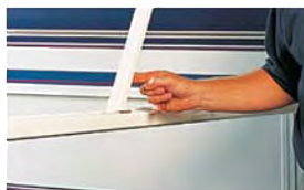
Single Track Slider for smooth sliding action without binding is standard on the Fiesta.
