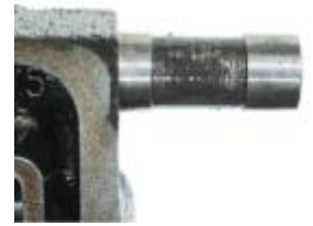
Valve body spool with heavy build up
