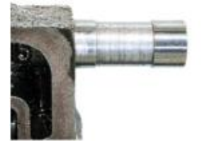
Valve body spool after transmission service
