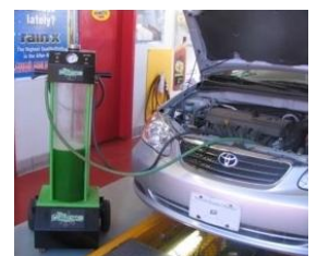
Coolant flush equipment
