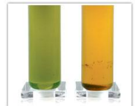
Clean vs. dirty, acidic coolant (antifreeze)
