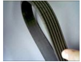
Worn accessory drive belt
