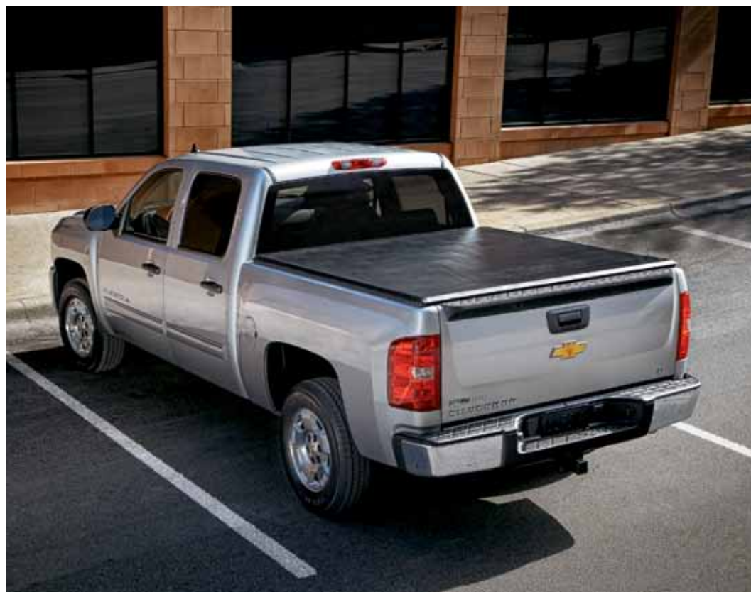
Silverado 1500 Crew Cab Short Box with XFE Fuel Economy Package, shown in Silver Ice Metallic. Silverado XFE features an aluminum block Vortec™ 5.3L V8, 6-speed automatic transmission, low-rolling resistance tires, aluminum wheels, soft tonneau cover and many other components designed to improve fuel efficiency.
