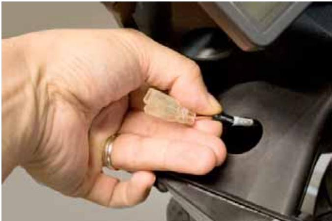
The 'ACC2' accessory power and ground wire can be found just underneath the 12-volt charging port cover on the KTM 1090 Adventure R.
