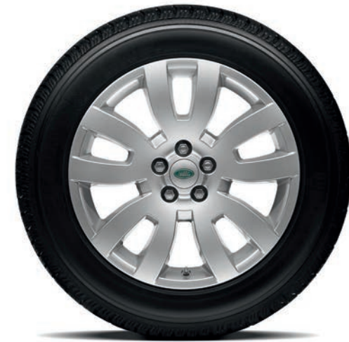
18-inch, 5-Split Spoke Alloy Wheel Sparkle Silver Finish LR002798 (315MHz) Tire size — 235/60 R18
