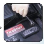
REMOVE THE OLD BATTERY – DO NOT TIP OR TILT THE BATTERY – Note the position of the battery terminals. Carefully lift out the battery and set it down on newspaper.
