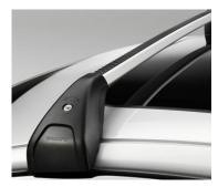
A specially designed transport system for loads on the roof. The load carriers are two swept aluminium profiles and feet with fully covering black plastic covers.
