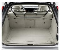
A practical protective grille that prevents loads or pets entering the passenger compartment in the event of heavy braking or a collision. It can be combined with a longitudinal divider to separate the truck area.
