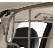
A practical protective grille that prevents loads or pets from being thrown forward into the passenger compartment in the event of heavy braking or a collision. It can be kept in either a raised or lowered position.
