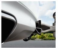
Integrated into bumper to keep maximum ground clearance hidden with a stylish cover when not in use. Wired into the all-wheel drive and traction control systems to provide maximum traction and correct sway due to crosswinds or evasive manoeuvring.
