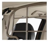
A practical protective grille that prevents loads or pets from being thrown forward into the passenger compartment in the event of heavy braking or a collision. It can be kept in either raised or lowered position.
