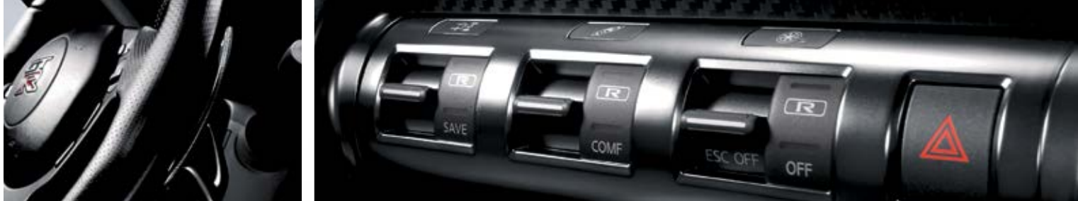
Steering-column-mounted paddle shifters Transmission settings: R-Mode, Normal and Save
