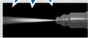
IMPROPERLY FUNCTIONING INJECTOR
