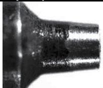
Diesel injector pintle after service
