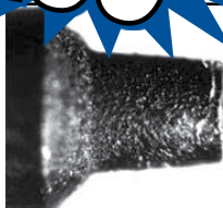
Diesel injector pintle before service
