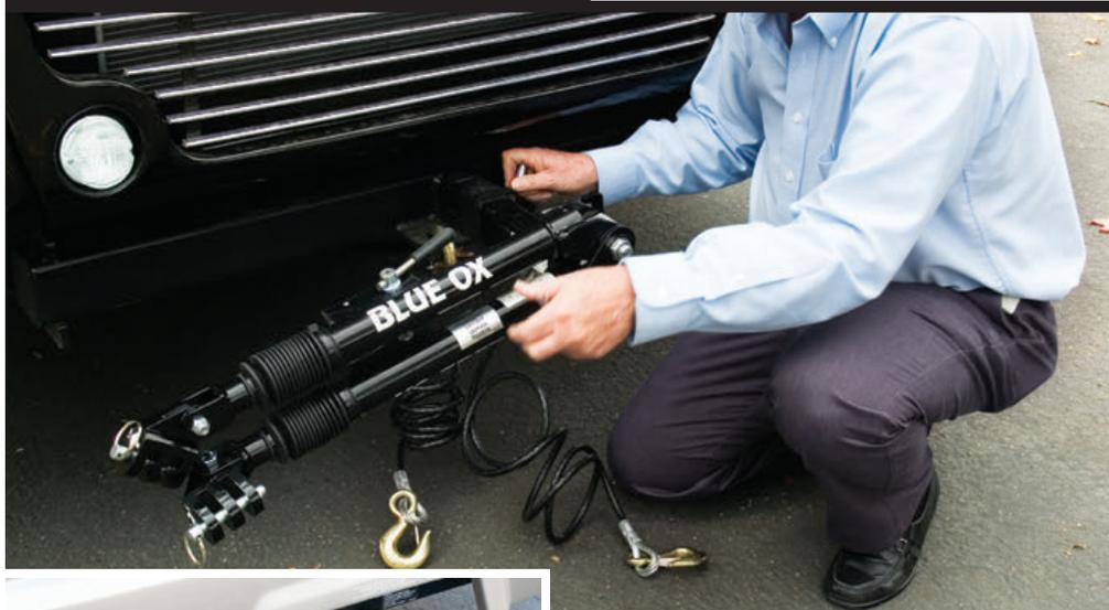
Above: Once the tow bar is pinned in the hitch receiver, make sure electric connections and safety cables are secure. Left: While driving your dinghy, this type of tow bar remains on the coach, out of harm's way.
