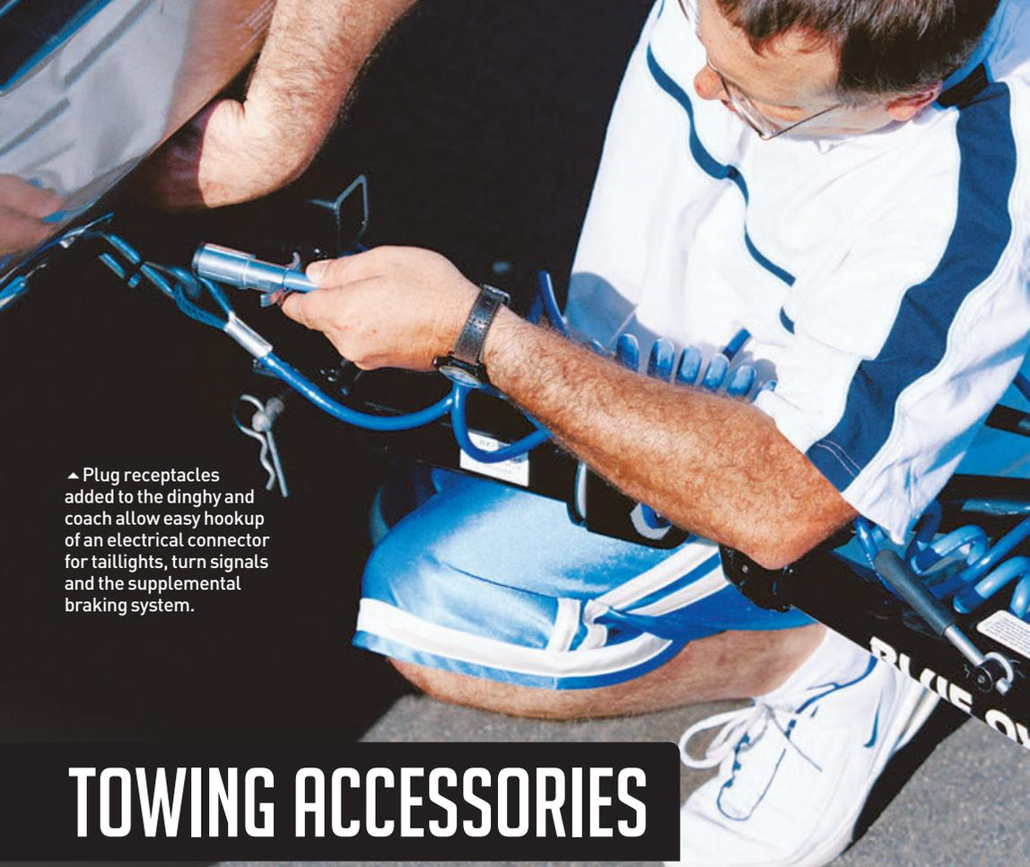
▲ Plug receptacles added to the dinghy and coach allow easy hookup of an electrical connector for taillights, turn signals and the supplemental braking system.
