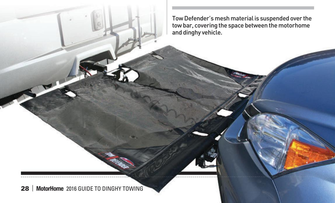
Tow Defender's mesh material is suspended over the tow bar, covering the space between the motorhome and dinghy vehicle.
