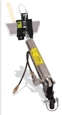
nected between the motorhome and dinghy. The hose runs through a small air reservoir installed under the hood, then runs to a brake actuator installed on the driver's seat floor, which then clamps to the brake pedal. The removable actuator has a quick-disconnect air line. A breakaway system is included.
