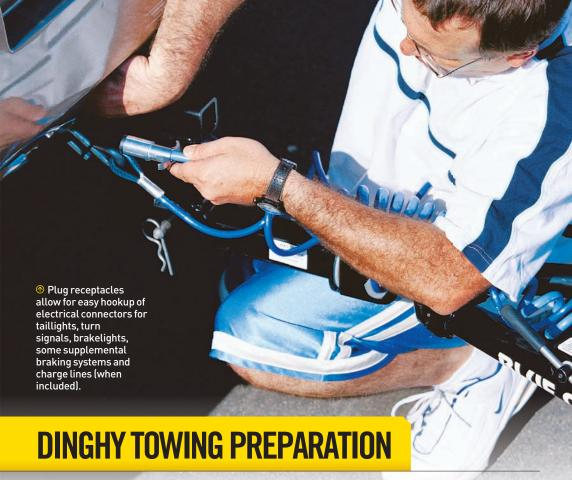
SAFE TOWING REQUIRES PROPER EQUIPMENT AND INSTALLATION
