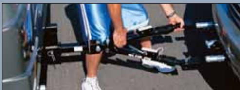
To hook up using a telescoping tow bar, the dinghy vehicle only needs to be near the center and midlength of bar.
