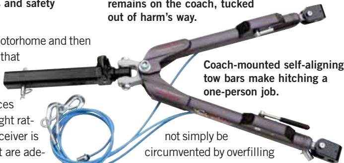
Coach-mounted self-aligning tow bars make hitching a one-person job.
